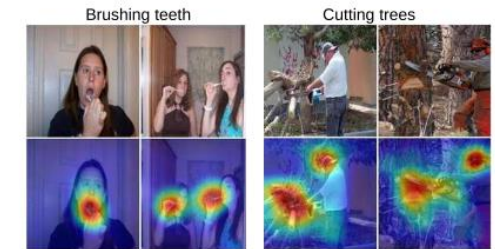
Figure 1. A simple modification of the global average pooling layer combined with our class activation mapping (CAM) technique allows the classification-trained CNN to both classify the image and localize class-specific image regions in a single forward-pass e.g., the toothbrush for brushing teeth and the chainsaw for cutting trees .
